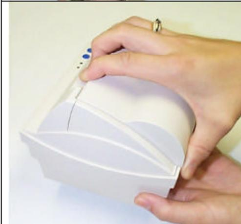
Option #2. Hold the base of the E-3202 in one hand. Using the other hand, place your thumb against the back of the paper bay door. Using your fingers on the front edge of the paper bay door, pull the door open.
